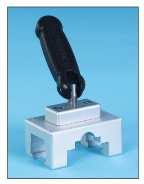
Deluxe Rail Clamp attaches anywhere along surgical table side rail. It accepts both 5/8" (1.6 cm) diameter round mounting posts and 1" x 3/8" (2.5 cm x .95 cm) flat bar mounting posts. Holds accessories in vertical or horizontal position.
