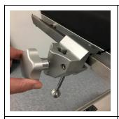
**Step 1.** *Place clamp onto rail (as shown).*
